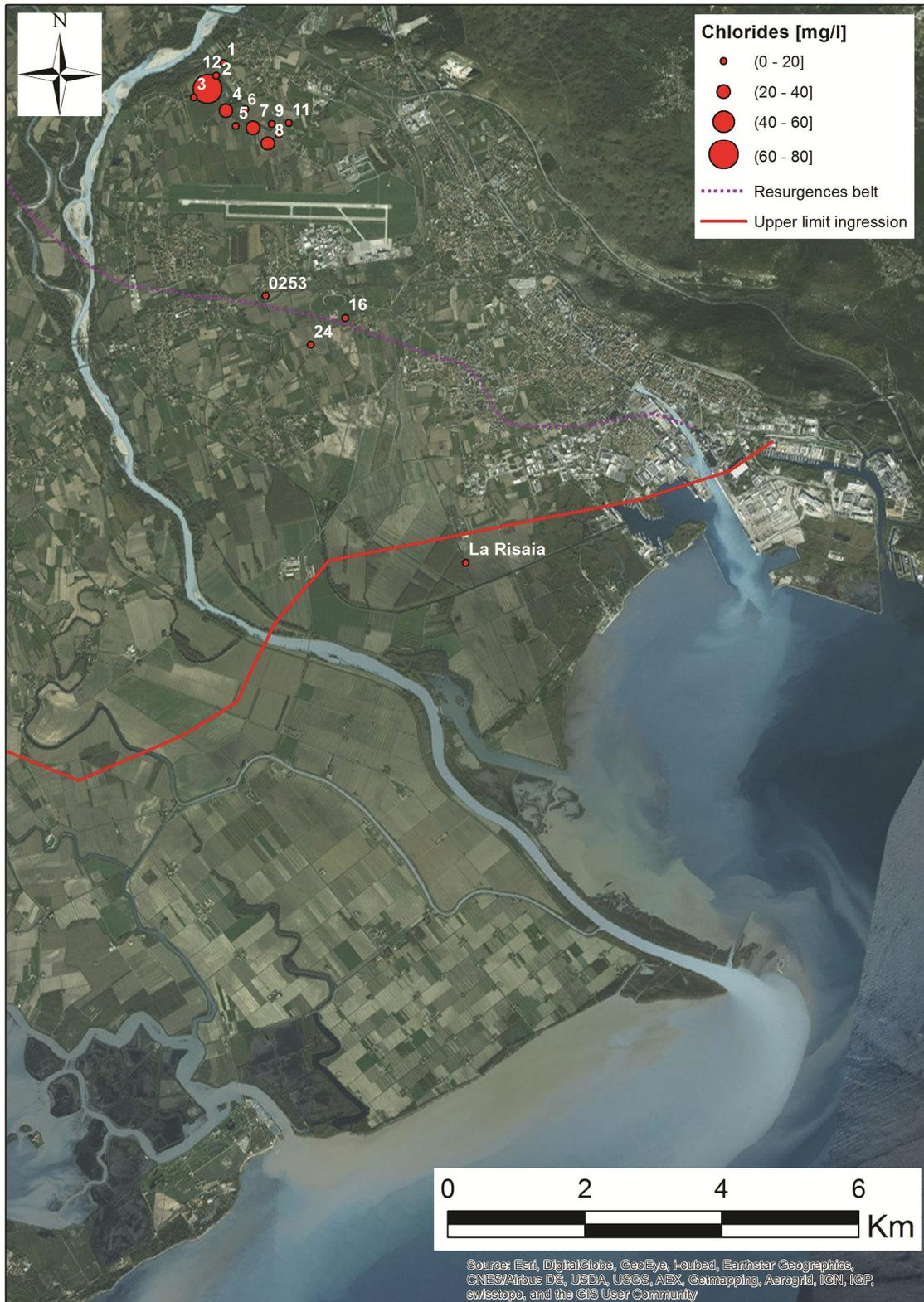
Figure 18: Chloride concentration evaluated for the surface and groundwaters. The red line represents the maximum ingression of the salt wedge measured in correspondence of the surface waters (rivers and channels).
