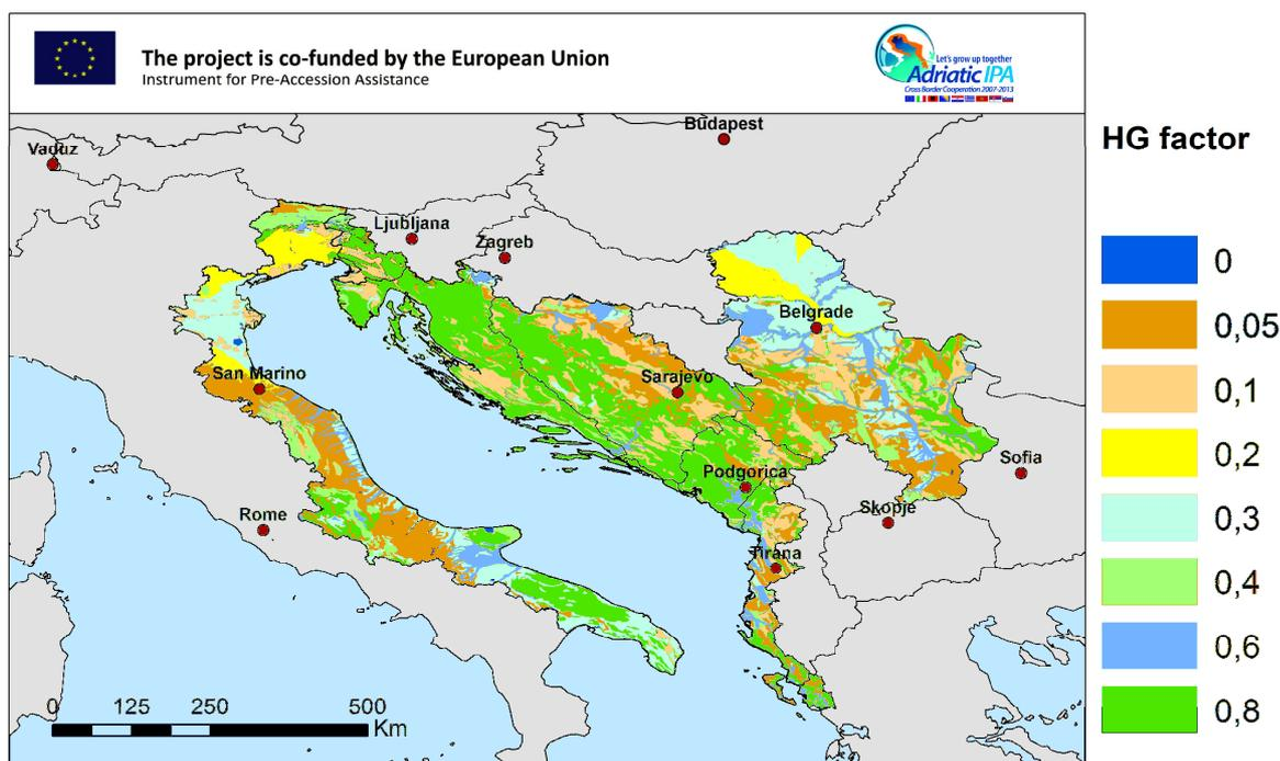
**Figure 27: Effective infiltration coefficient as HG factor.**
