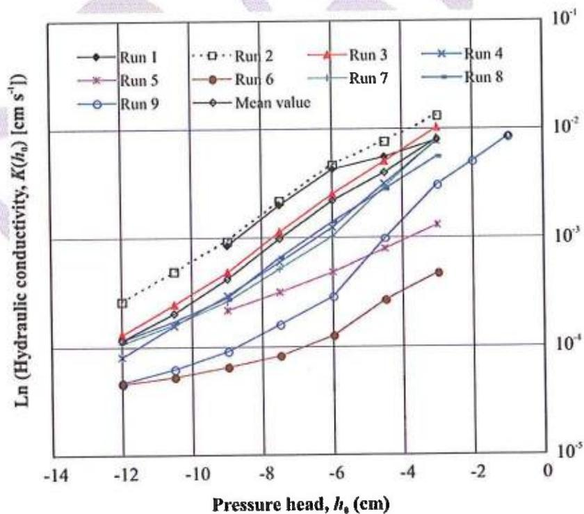
Fig 4.2.4. Soil hydraulic conductivity  $K(h_0)$  versus pressure head  $h_0$ .
